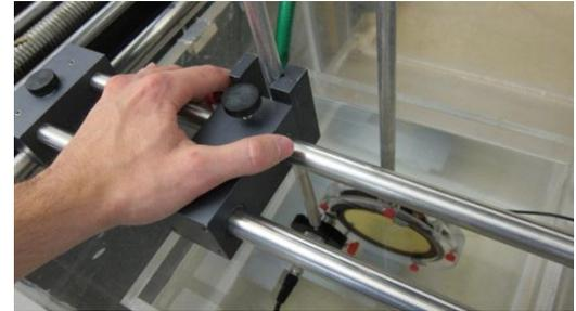
A. Secure the metal rod with the transducer to the sliding clamp on the rail above the Daedal tank. Make sure to align the face of the transducer with the ring. They must be parallel. If they are not parallel it will be impossible to find symmetry around the focus.
