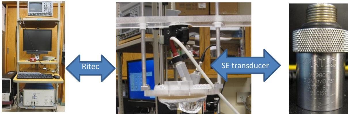
Many BRL experiments use a single element transducer with the Ritec system, as illustrated in the upper middle photo. It is usually desired to know the spatial pressure levels produced from an ultrasound device for the experimental design. Therefore, a calibration is performed. BRL SE transducers are designed to transmit through biological tissue. Since tissue is mainly comprised of water, the SE transducers are impedance matched to water and calibrations are done in water.
