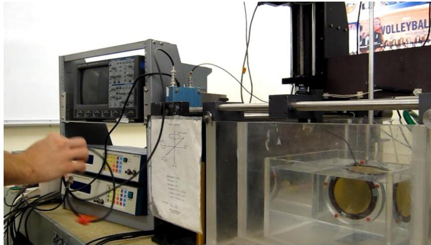
Use the cable which came in the hydrophone case to connect the output of pre-amp to the input channel of the daedal.
