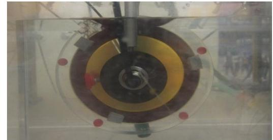
B. Slide the transducer to an edge of the hydrophone. Rotate the transducer to make sure it is parallel with the hydrophone. The transducer should be approximately centered along axis three in reference to the hydrophone and over the active element.
