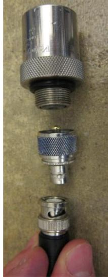
B. Attach the transducer-to-BNC adaptor found on the Ritec cart. Connect the Ritec "To Transducer" cable.
