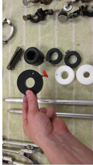
C. Set the transducer in an appropriate sized holder ring off of the daedal accessory table in the Daedal room. Make the screws finger tight. Screw in an aluminum rod to the holder ring.
