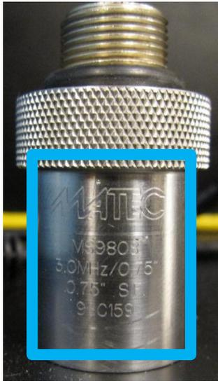
A. Record the transducer properties. Write down the serial number, model number, frequency and focal length/diameter) of the transducer as well as the date of the scan.
