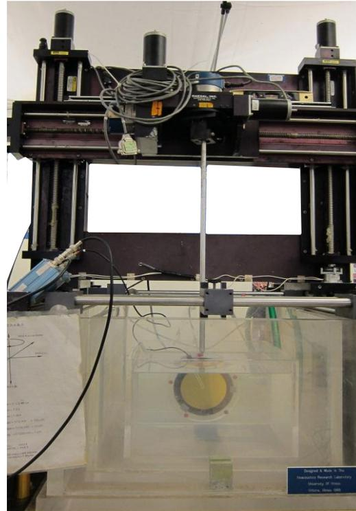
**A. Set up one of the Marconi hydrophones with accompanying pre-amplifier (Refer to the Hydrophone manuals for detailed instructions).**
