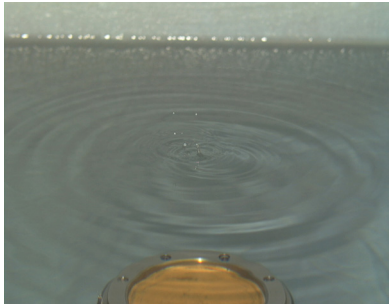
Figure 3.7 Water-Air Boundary Broken at Threshold
