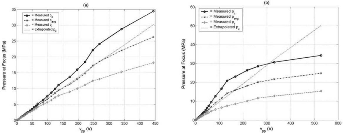
Figure 2: Direct comparison of pressures at the focus. (a)  $\sim 5.5$  MHz  $f\#$  of 1 transducer (b)  $\sim 5.5$  MHz  $f\#$  of 2 transducer
