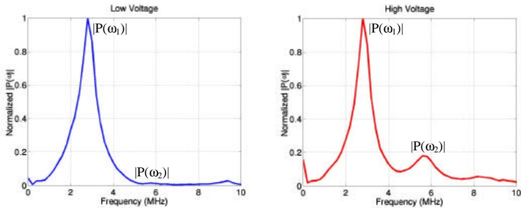
Figure 4.1: Typical frequency spectrum at the focus of a spherically focused transducer under two different drive conditions.
