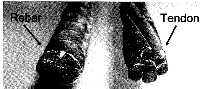
Figure 1.10: Photograph of rebar (left) and seven-wire strand (right). Rebar was monitored in this report.
