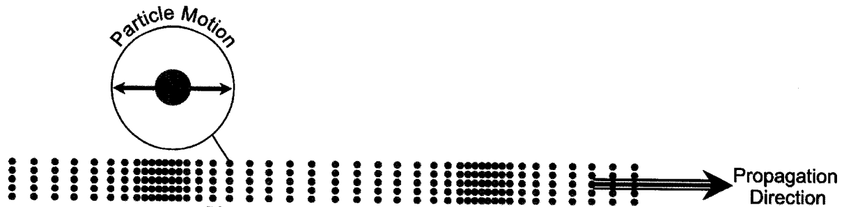
Figure F.3: Compressional propagation in a bulk medium.
